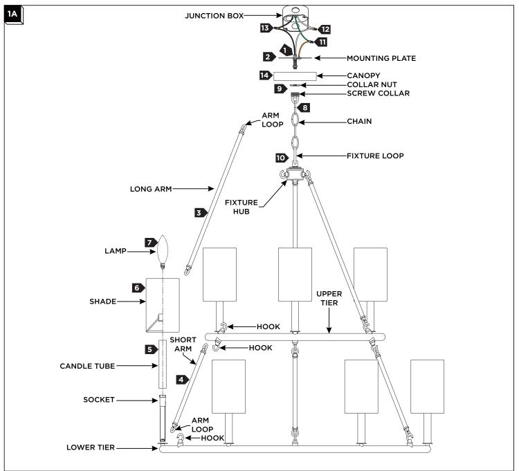
If necessary, screw the short end of the threaded nipple onto the mounting plate, then screw the screw collar and canopy loop onto the threaded nipple.
